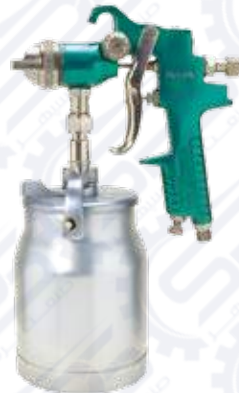
★★GS-212S Spray Gun, HVLP Option Nozzles : 1.0, 1.2, 1.4, 1.7, 2.0, 2.3 mm Working Pressure : 30 ~ 43 psi (2 ~ 3 bar) Cup : 1.0 L Weight of Gun : 0.63 kg Fluid Inlet : 3/8"
