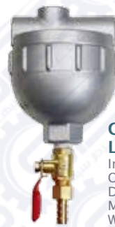
GS-15 Paint Regulator Inlet Size : 1/4" Output Size : 1/4" Max Working Pressure : 90 psi ( 6.2 bar) Regulated Pressure : 0 ~ 35 psi (0 ~ 1.3 bar) Max Delivery : 2.4 l/min Weight : 760 g
