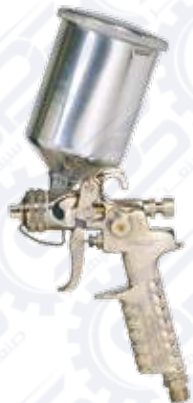
★★GS-206G Mini Spray Gun, HP Option Nozzles : 0.5, 0.8, 1.0, 1.1, 1.2 Working Pressure : 1.5 mm Working Pressure : 38 ~ 60 psi (2.6 ~ 4 bar) Air Consumption : 132 l/min Cup : 125 ml Weight of Gun : 0.3 kg Fluid Inlet : 1/4"
