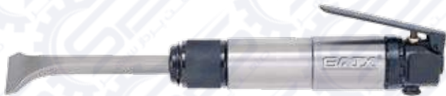
★★★★GP-0318 Air Flux Chipper Free Speed : 4,000 bpm Stroke : 34 mm Air Consumption : 400 l/min Length : 375 mm Weight : 2.6 kg
