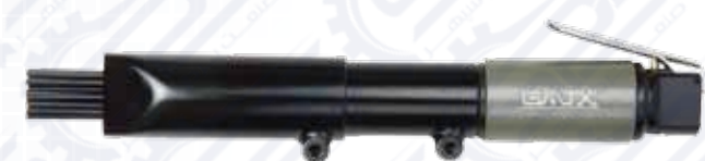
★★★★GP-0326 Air Needle Scaler Free Speed : 3,700 bpm Needle Size : \Phi 3 x 180 mm x 19 pcs Length : 375 mm Weight : 2.6 kg
