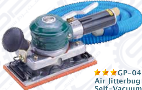
★★★★GP-0428 Air Jitterbug Sander Free Speed : 7,000 rpm Pad Size : 93 x 176 mm Orbital : 5 mm Air Consumption : 400 l/min Air Pressure : 90 psi ( 6.2 bar) Net Weight : 1.9 kg
