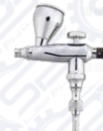
★★★GS-731 0.3 mm Regulated Air Brush Working Pressure : 15 ~ 30 psi (1 ~ 2 bar) Cup Capacity : 7 cc
