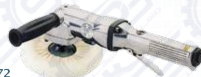
★★ GP-0472 7" Angle Polisher Free Speed : 2,500 rpm Pad Size : 7" Spindle Thread : 5/8"-11,M14 Air Consumption : 450 l/min Air Pressure : 90 psi ( 6.2 bar) Net Weight : 2.25 kg
