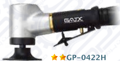
★★GP-0422H 3" Angle Sander Free Speed : 18,000 rpm Power : 0.45 HP (0.34kw) Air Consumption : 480 l/min Net Weight : 0.96 kg ■ Gearless
