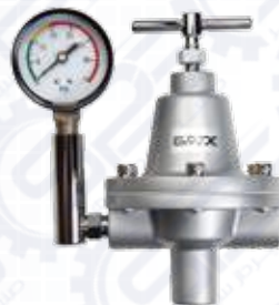
GS-15 Paint Regulator Inlet Size : 1/4" Output Size : 1/4" Max Working Pressure : 90 psi ( 6.2 bar) Regulated Pressure : 0 ~ 35 psi (0 ~ 1.3 bar) Max Delivery : 2.4 l/min Weight : 760 g
