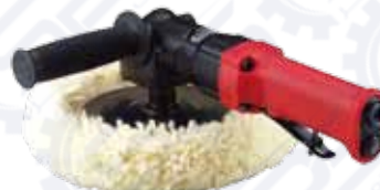
★★★★GP-0412 127~203 mm Angle Sander Free Speed : 0~2,500 rpm Pad Size : 125 mm ~ 203 mm Air Consumption : 85 l/min Air Pressure : 90 psi ( 6.2 bar) Net Weight : 2.0 kg Packing : 23.5 kg/ 1.9 cft/ 10 pcs
